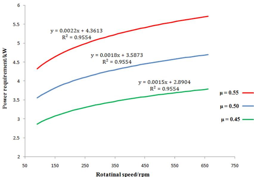
Figure 7 Effect of manure-manure friction and rotational speed of auger on PTO power requirement
