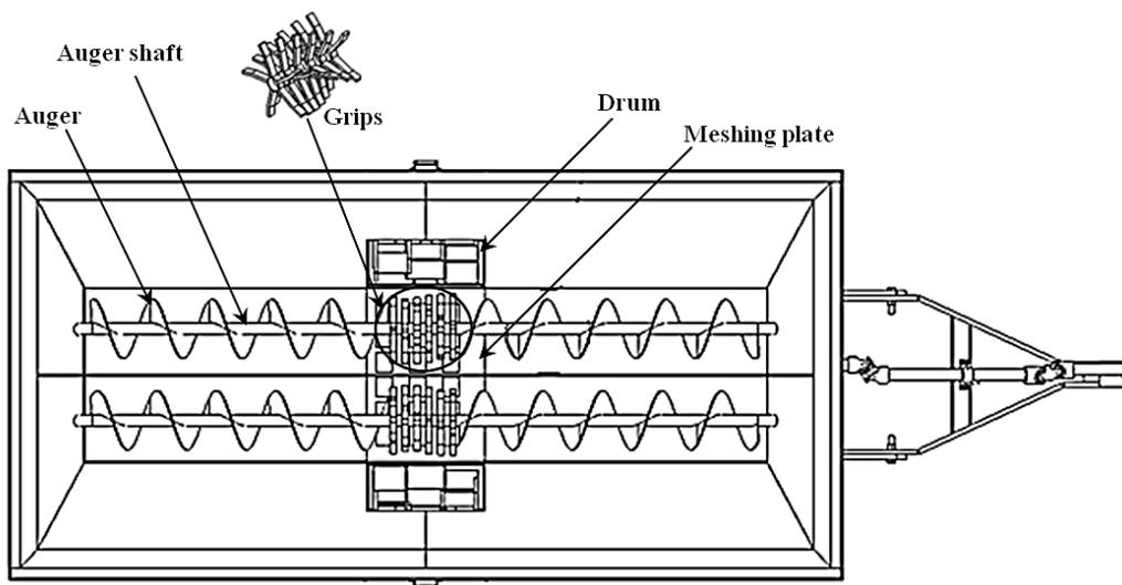
Figure 2 Top view of helical wet manure distributor and its component
