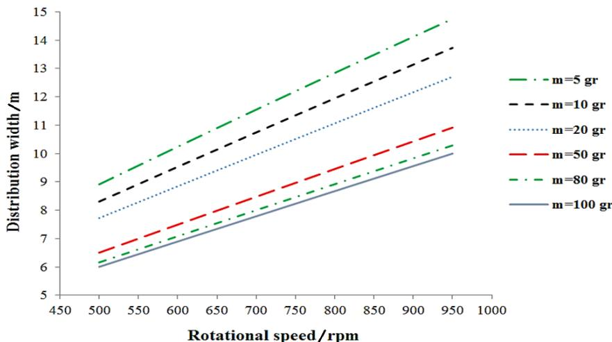
Figure 6 Effect of drum speed and particle mass of manure on distribution width of machine
