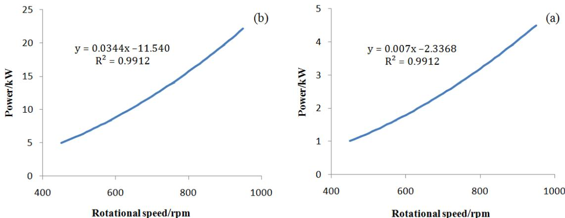
Figure 8 Effect of rotational speed of drums on power requirement for (a) idle rotational speed of drums and (b) spreading of manure
