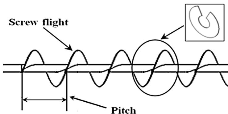
Figure 3A schematic diagram of a screw conveyor
