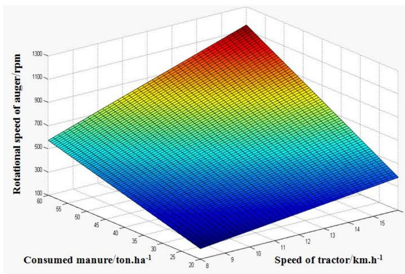
Figure 5 Effect of tractor’s forward speed and amounts of manure application on the rotational speed of auger
