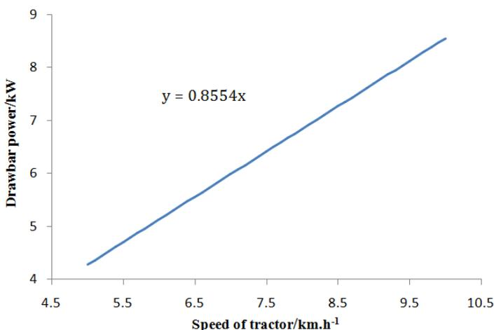
Figure 9 Effect of speed of tractor on drawbar power
