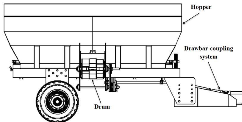
Figure 1 Side view of helical wet manure distributor
