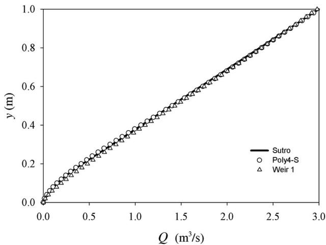
Fig. 1. Comparison with nonlinear domain of the Sutro weir
