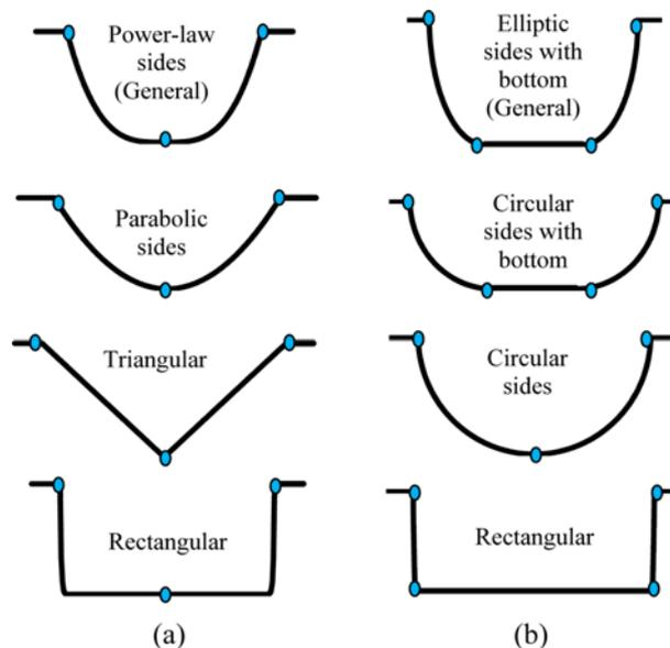
Fig. 1. Comparison of the Special Cases of The Proposed and Power-Law Sections: (a) Power-Law Section, (b) Elliptic Section
