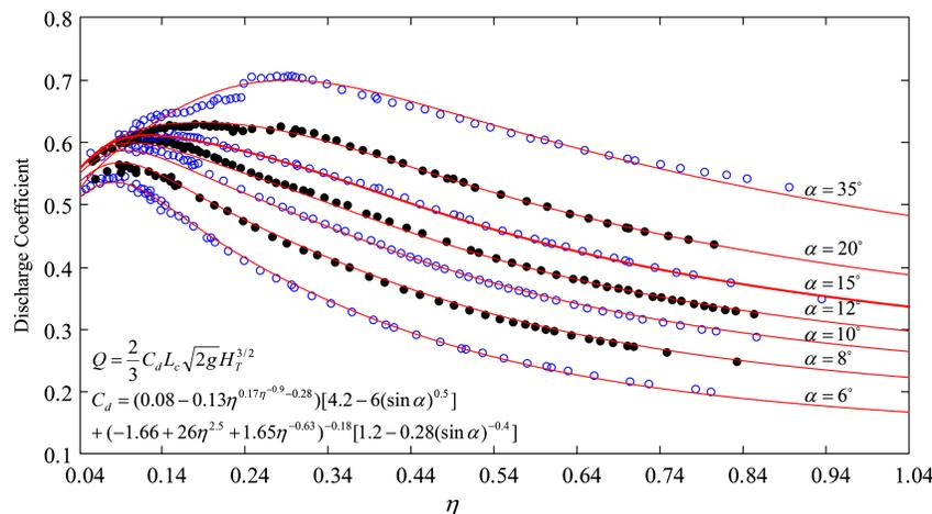
Fig. 1. Variation of discharge coefficient of quarter-round trapezoidal labyrinth weirs with head to weir height ratio ( $\eta$ ) for different sidewall angles
