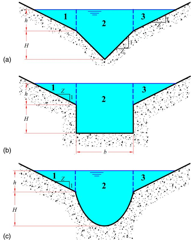
**Fig. 1.** Compound channels with nonzero lateral slopes and their subsections: (a) compound triangular section; (b) compound rectangular section; (c) compound parabolic section
